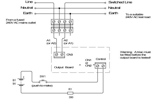
Test circuit for the output board
