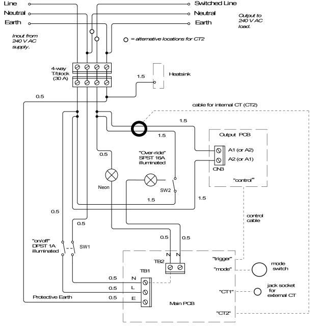
NB. Mains wiring is shown with solid lines, the recommended CSA is shown in mm2. Low-voltage wiring is shown with dotted lines.
